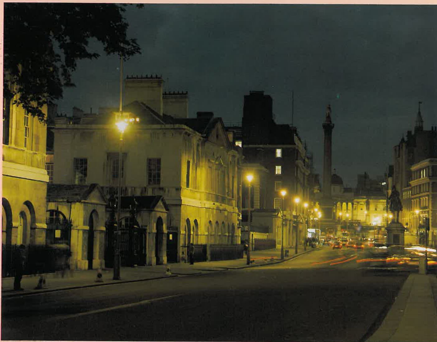
In Curzon Street, (below) existing lanterns originally housing 1,000W incandescent lamps were replaced by 400W SON, as were those outside the Horseguards in Whitehall shown above.
